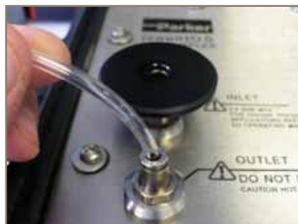
Attach OUTLET (Ø 4mm) hose
