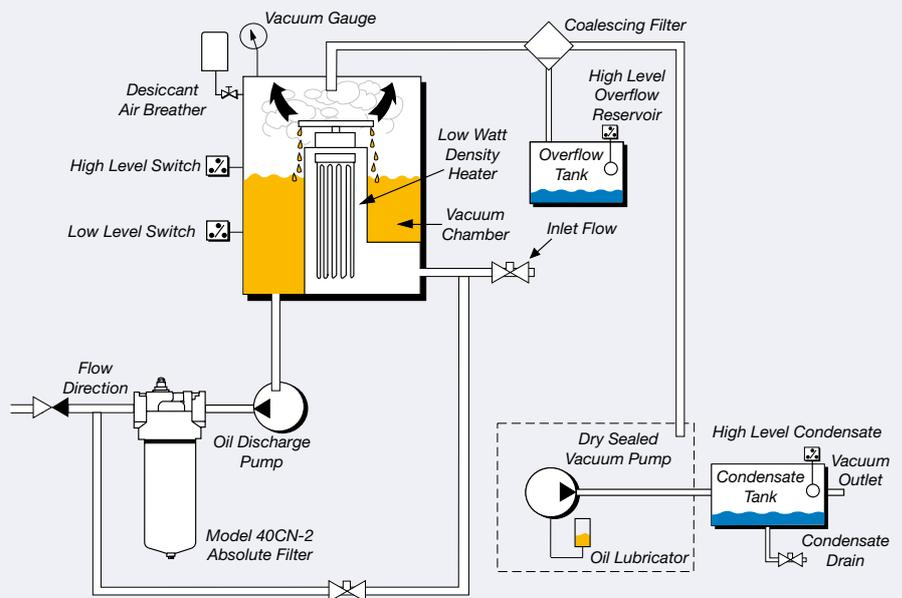
Contaminated fluid is drawn through the Sentinel circuit by vacuum. The fluid is subjected to optimum vacuum, temperature and surface area to reduce the boiling point of water and convert water to water vapour. Optimum temperature is achieved with a low watt density heater. Maximum surface area is accomplished by passing the fluid through a unique diffusing column.
