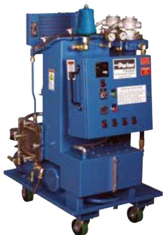
The maximum flow for the PVS 2700 model is 170 l/min and the PVS 600 model shown above is 38 l/min.
